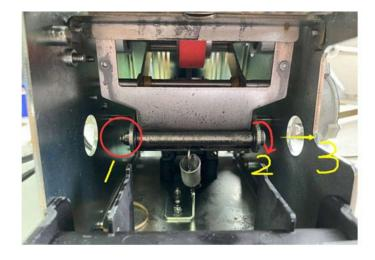
• Pull out the heating device to take out the cutter, as shown in the attached figure
