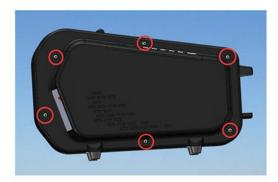
• Remove the pressing plate on the display screen, as shown in the attached figure
