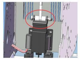
• Replace the electromagnet with a new one
