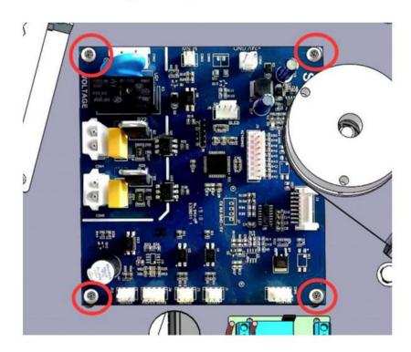
• See the attached figure for the description of wiring on the circuit board
