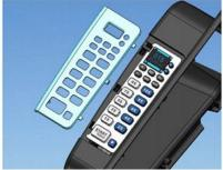
• Remove the display screen and the silica gel key, as shown in the attached figure
